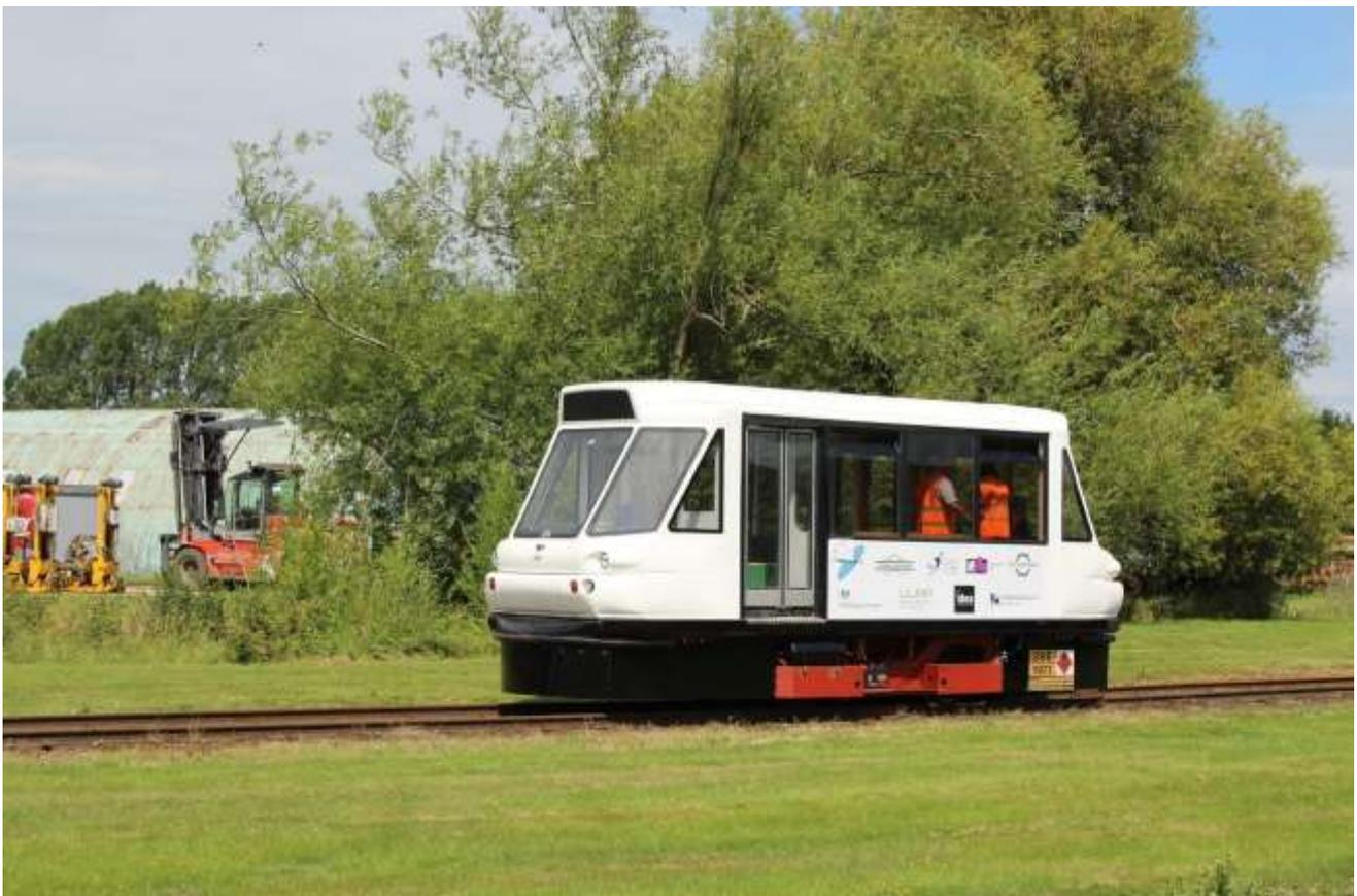
Testbed railcar undertaking trial running at the Rail Technical Centre at Long Marston, Warwickshire, on 22nd July, 2020. The red coloured section of underframe houses the bogie-length driveline mechanism.
