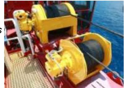
Air motors can be very simple with long service intervals and are more straightforward to maintain than other rotary engines.
