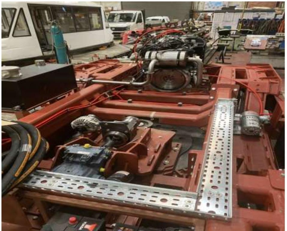
*The First of A Kind testbed chassis at Severn Lamb's factory almost ready for integration with the body (above left) at the point when the factory was locked down due to the Coronavirus pandemic.*
