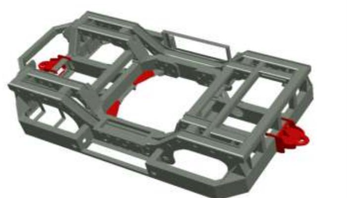
Special framework designed to house the traction driveline for a fully integrated bogie
