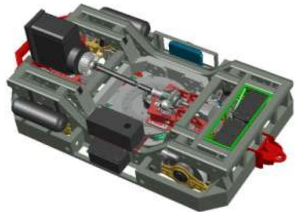
3D CAD image of bogie frame with primary and secondary drivelines and energy-storing flywheel
