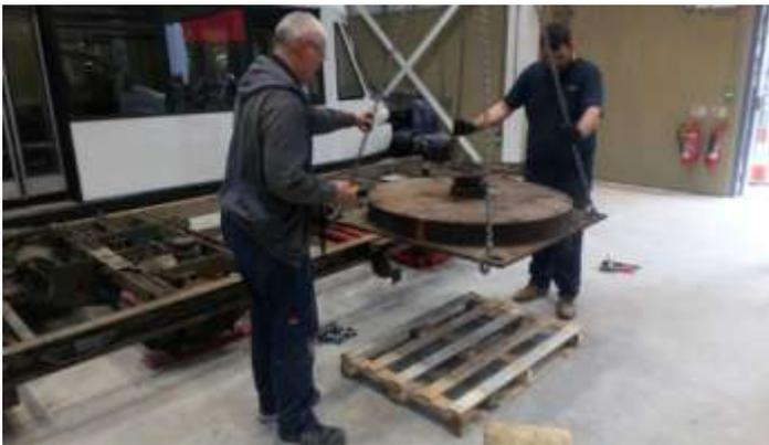
*Following removal of body from chassis using the workshop's 10t crane., flywheel extracted for overhaul*
