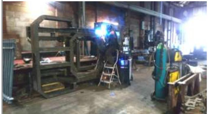
Cradley Heath welders, Oakham Fabrications, at work building the first prototype bogie frame
