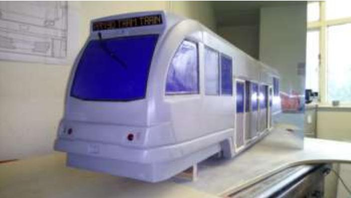
Wooden mock up of a 90 passenger vehicle with provision for installing bogies at each end
