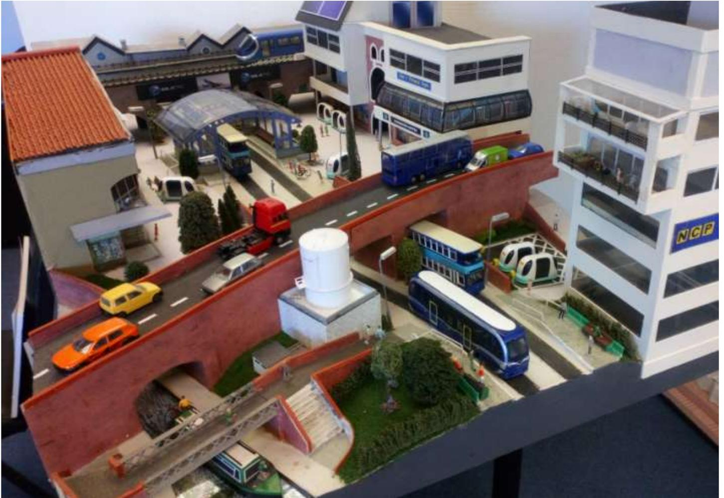
The Clear Air Zone model illustrates a 'cascade' of transport amenities with, at the top, a fast metro service linking to a cross town tramway, then to 'CAV' (Connected Autonomous Vehicles 'pods') A conventional highway crosses the 'zone' by means of an overpass with provision for buses to drop off passengers and motorists to park their cars at the edge of the zone.
