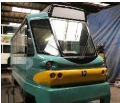
*Photographed in September 2018 after the body was re-united with its re-engineered chassis, the Class 139 prototype 'Car 12' appears pretty well ready to return to public service*
