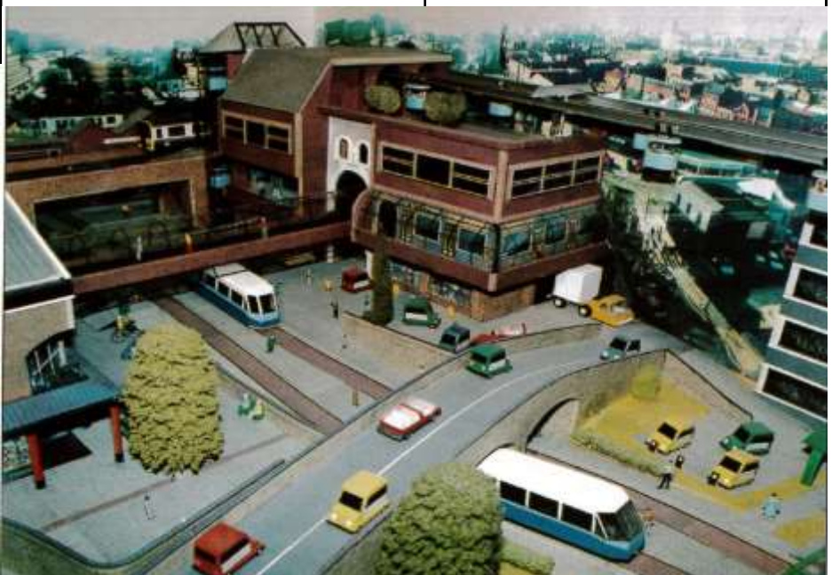
A special model was designed and built for the 1990s Technology Foresight Transport Panel to illustrate the concept of a pollution free, Clean Air Zone established in the central area of a Town or City. The model comprises various means by which workers and visitors can move around in nil emission mode. Technologies include small 'pod'-type vehicles, electric vans and a small tramway connecting the station at the top left of the model with other locations in the town.
