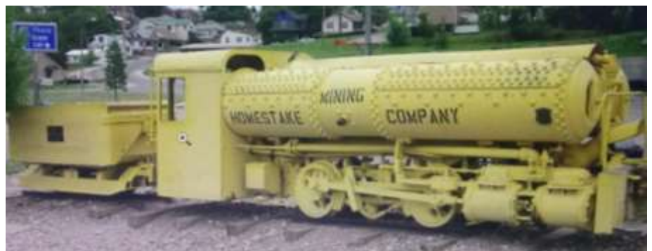
For much of the previous century the mining and tunnelling industry in the United States used compressed air locomotives for hauling iron ore trains underground.
