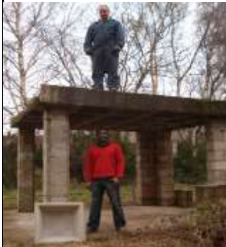
After the Mozambique flood disaster a new high & dry technology for flood refuges was tested in Cradley Heath then introduced in the field. Reference structure demolished
