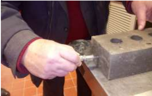
Using a soil penetrometer in order to assess the 'green' strength of a low carbon brick made with the new type of binder using manufacturing equipment supplied by Parry Building Products.
