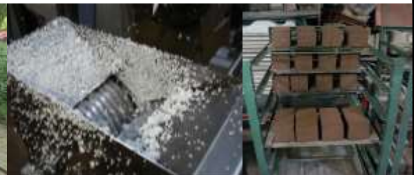
New technology incorporating particles of expanded polystyrene waste into concrete to produce lightweight bricks terminated because equipment scrapped
