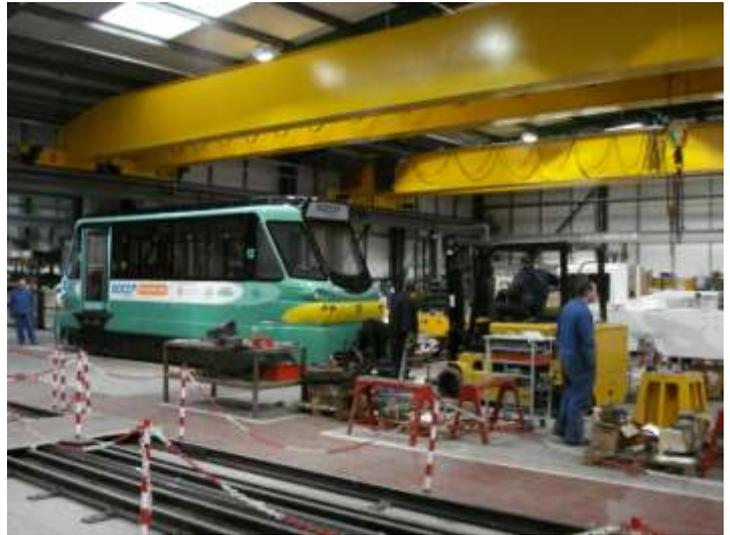
*PPM railcar 139000 in 2012 at Clayton's works for removal of its body for engineering examination after a transmission failure during commissioning trials.*
