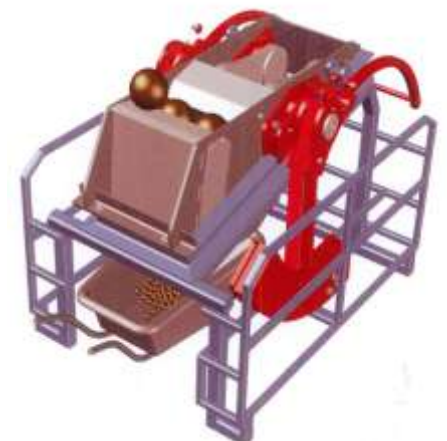
Computer-generated image of a kinetic energy assisted manual stone crusher, using heavy swinging pendulums
