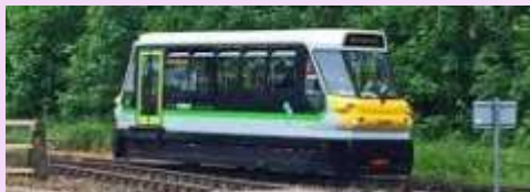
With clean, quiet gas hybrid propulsion the Class 139 will adapt readily to street running applications.
