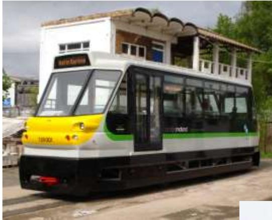
*Left: Photographed in 2009 prior to departure from PPM's Cradley Heath base Class 139 railcar 139001 has now operated in service for 5 1/2 years proving the performance and serviceability of the flywheel hybrid traction system.*
