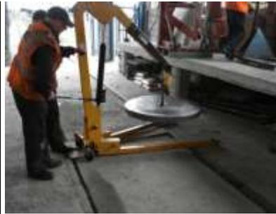
*Class 139 flywheel having just been removed to be sent for overhaul and rebalancing.*
