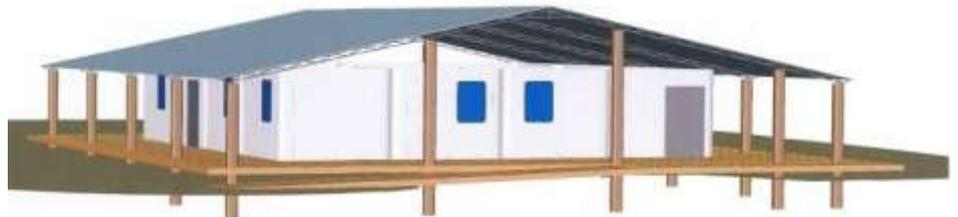
*Concept of High & Dry raised concrete platform with sheet roof. The internal structure made up of prefabricated panels designed for ease of cleaning*
