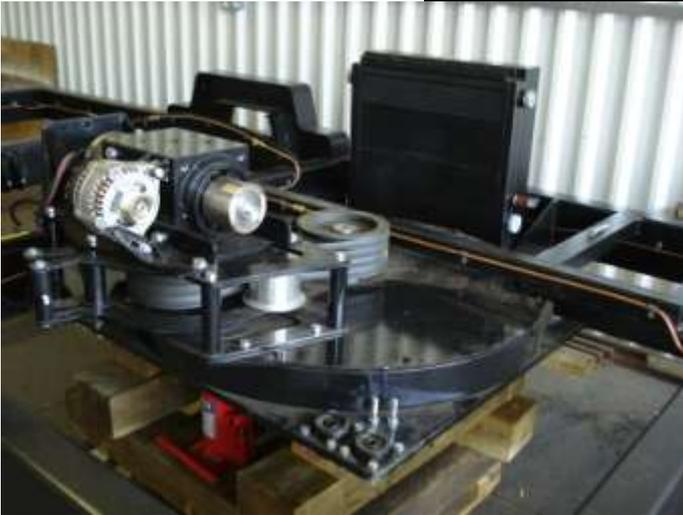
Engine, bevel gearbox and flywheel mounted on a sled or raft for ease of installation.
