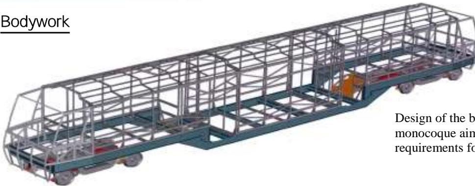
Design of the body framework is as a semi-monocoque aiming to meet the structural requirements for UK tram-trains
