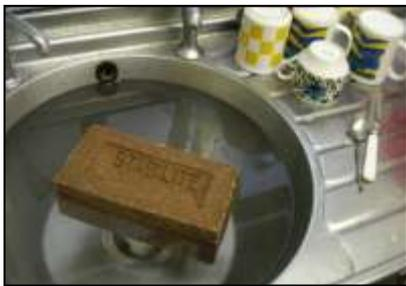
**With the correct processing & particle grading a new type of impermeable concrete can be produced which floats on water**
