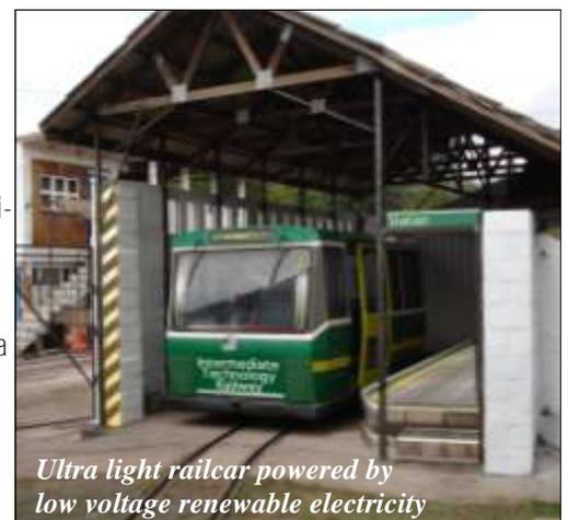
**Ultra light railcar powered by low voltage renewable electricity**
