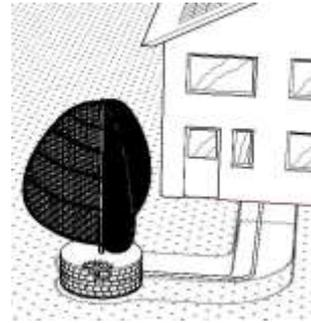
The money tree rotating slowly and safely on a vertical shaft will accumulate energy into store. Using high gearing it will run a compressor manufacturing high pressure air supplying a 'hot' feed and a cool feed to the building. Release of air under pressure will also operate a low watt electricity generator for LED lighting in the adjacent building. Heat, cold and power cost money.
