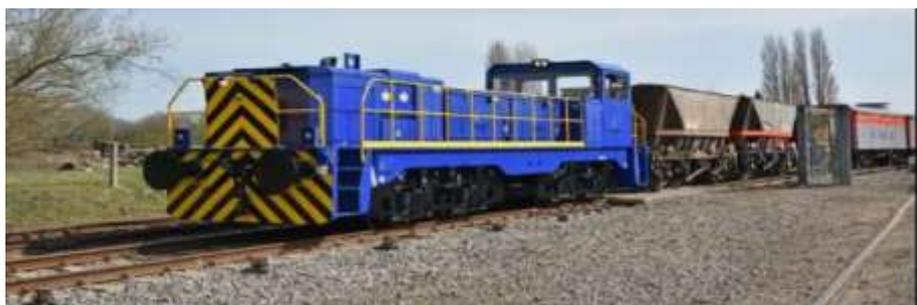
*One of a batch of five Clayton 90t hybrid locomotives under trial at Chasewater Railway where PPM have also historically commissioned their hybrid railcars.*
