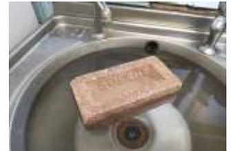
A brick so light it can hang on a piece of cotton and one which floats on water
