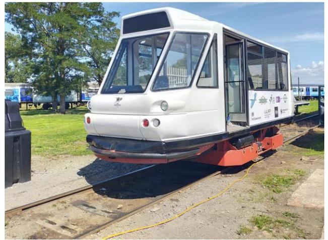
20 years later at Long Marston, Sustraco's railcar is back in action as a 'First of A Kind' containing the complete driveline within the frame of a train bogie opening the way to building larger vehicles.
